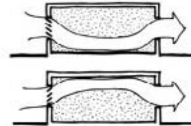
Louvres can direct airflow upward or downward.
