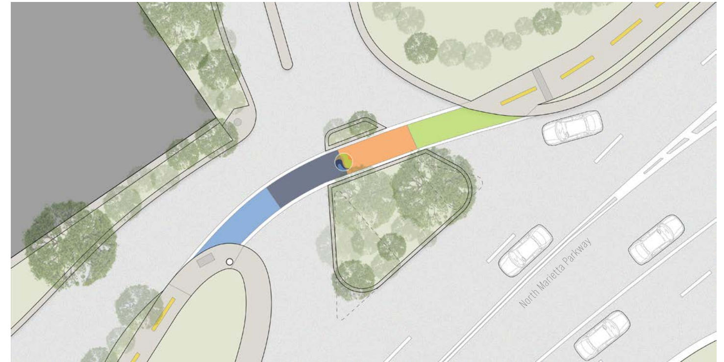
Option 2 - Intersection redesign with crosswalk to trail realignment and navigation improvements.
