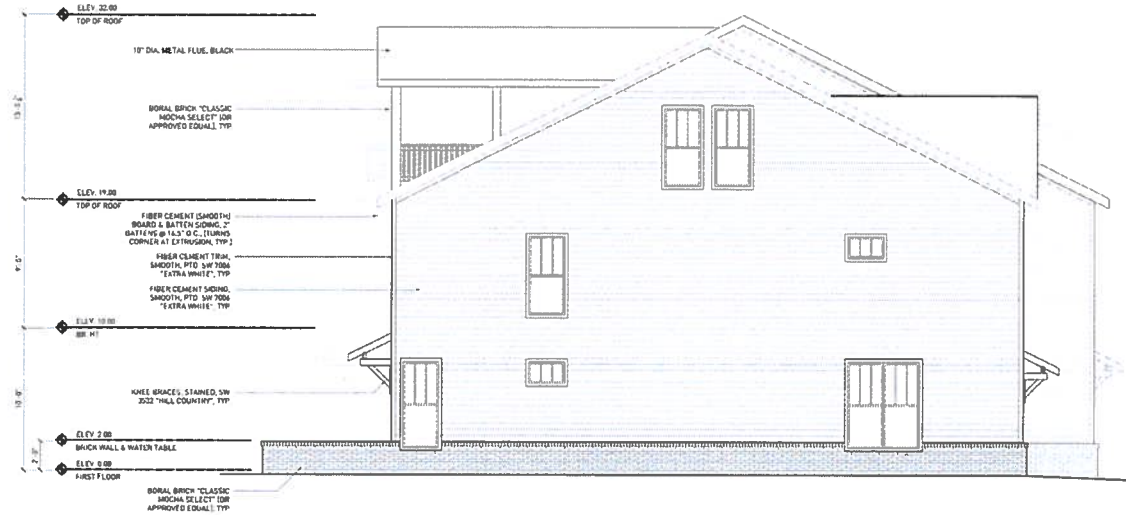
2 NORTH ELEVATION (UNITS 13-15) SCALE: 1/4" = 1'-0"
